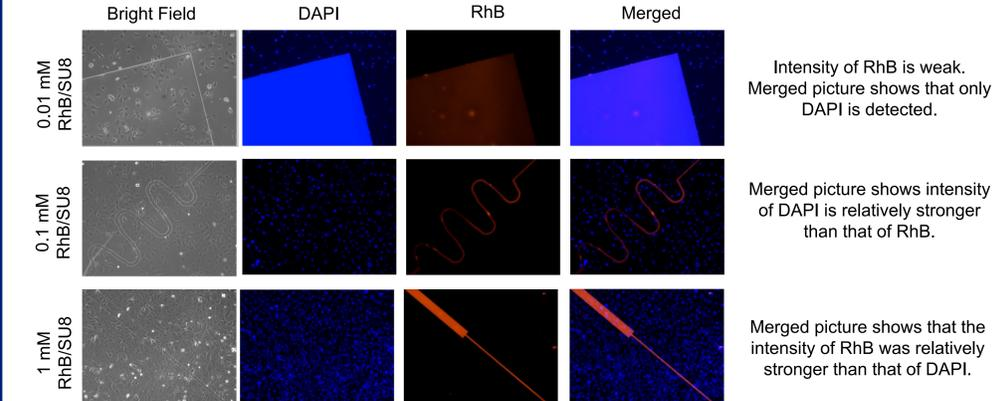
Upon comparing the fluorescence intensities of DAPI and Rhodamine B (RhB), it was determined that the appropriate concentration range for RhB/SU8 is between 0.1 mM and 1 mM. This range ensures that the fluorescence intensity of RhB/SU8 matches that of DAPI, allowing for optimal imaging and accurate visualization of the interface.
