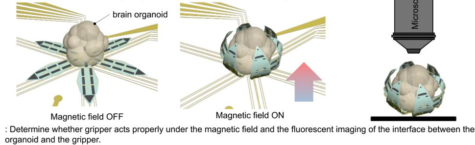
Determine whether gripper acts properly under the magnetic field and the fluorescent imaging of the interface between the organoid and the gripper.
