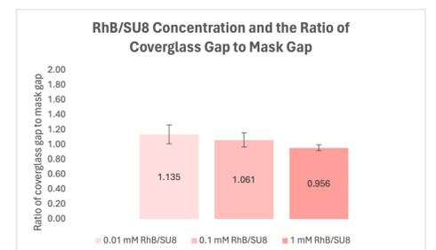
A ratio closer to 1 indicates that the lithography was performed well and that the lithography conditions were appropriate. The ratios for 0.01 mM RhB/SU8, 0.1 mM RhB/SU8, and 1 mM RhB/SU8 were all close to 1, confirming the suitability of these conditions.
