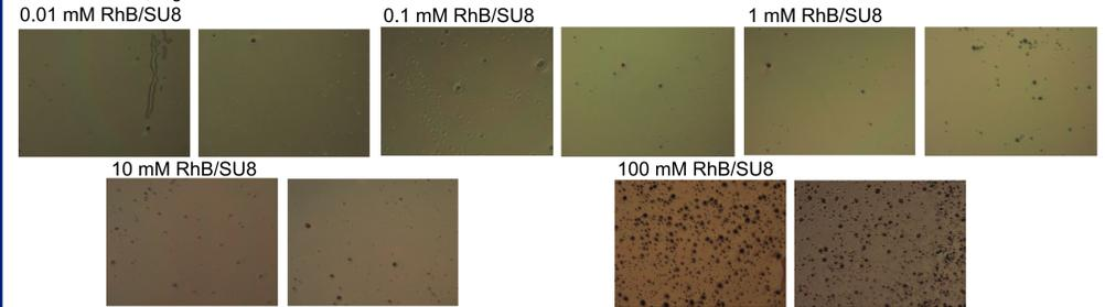
Samples 10mM and 100mM exhibited a large number of dye particles on the surface, which could lead to improper lithography. In contrast, samples 0.01mM, 0.1mM, and 1mM appeared to contain an adequate amount of dye particles, warranting further examination.
