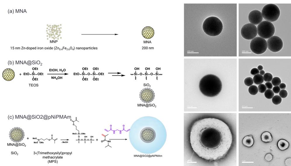
**Fig. 1.** Schematics and TEM images of (a) magnetic nanoparticle assembly (MNA) in a face-centered cubic (FCC) superlattice structure, (b) MNC@SiO<sub>2</sub>, and (c) MNC@SiO<sub>2</sub>@pNIPMAm. (left) a single particle, (right) a set of particles.
