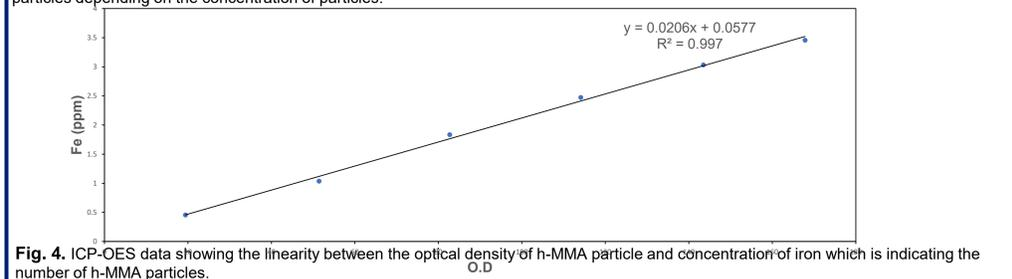
**Fig. 4.** ICP-OES data showing the linearity between the optical density of h-MMA particle and concentration of iron which is indicating the number of h-MMA particles.
