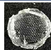
SEM image of one hexagonal pillar of PDMS. Could observe the depth of each well is over 100um
