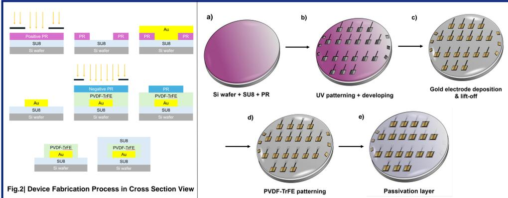
Fig. 2] Device Fabrication Process in Cross Section View
