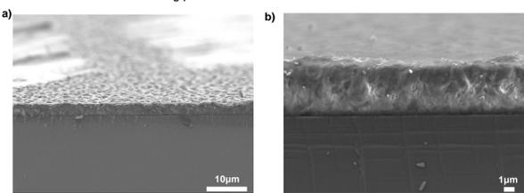
Fig. 6] SEM of PVDF-TrFE film deposited on Silicon Wafer. Side view of sliced wafer coated with PVDF with each conditions of a) MEK 8% w/v 1000rpm and b) MEK 10% 1000rpm.
