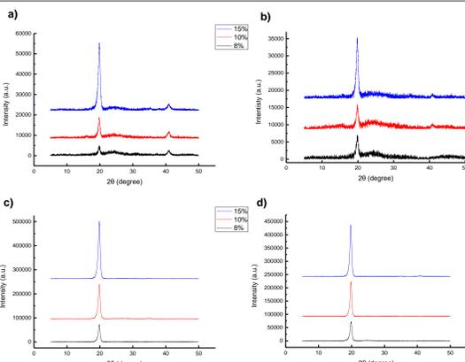
Fig. 4] XRD Results with different solvent type, spin coating rpm, solution concentration. a) DMF solvent spin coated in 1000 rpm, b) DMF solvent spin coated in 4000 rpm, c) MEK solvent spin coated in 1000 rpm, and d) MEK solvent spin coated in 4000 rpm. Peak values in 20 degrees show successful formation of  $\beta$  phases in all solutions.
