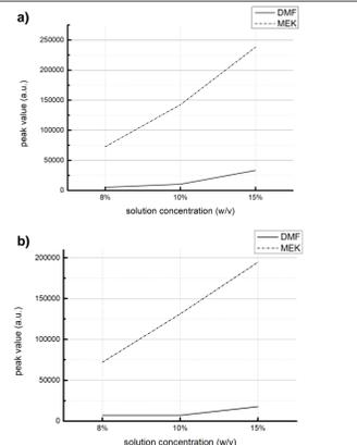
Fig. 5] Trend of peak value with different solution concentration. a) MEK and DMF spin coated in 1000 rpm and b) 4000 rpm. Peak value increases with concentration.
