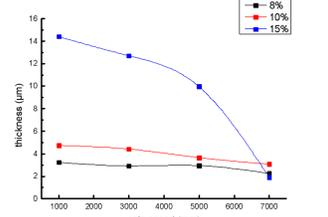
Fig. 7] Film thickness with different concentration and spin coating rpm. Thickness decreases with increasing rpm and shows a drop around 5000 rpm.
