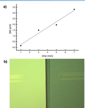
Fig. 10] Etching results of 10% 1000 rpm coated PVDF-TrFE solution in solvent MEK. a) Etching rate with recipe of O<sub>2</sub> 150W is calculated as 497 nm/min. (thickness (t)) b) Etching boundary picture. Left section is etched. Expected complete etching time for 10% w/v solution is calculated as 9.5 min. It is shown that microscale etching is possible via RIE.
