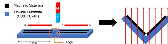
The magnetic actuation mechanism utilizes the basic characteristic of the magnetized materials to align in a specific direction according to their magnetization direction under the external magnetic field
